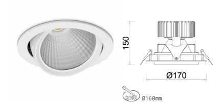
COB 3000 [K] CRI97 Light colour CRI Led chip flux 2402 [lm] Luminous flux 1921 [lm] System power 21 [W] Luminaire Efficiency 91 [lm/W] Beam angle 15° Controller ON/OFF MacAdam 3 SDCM
