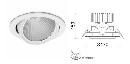
COB 3500 [K] PREMIUM WHITE Light colour CRI 90 Led chip flux 4038 [lm] Luminous flux 3230 [lm] System power 35 [W] Luminaire Efficiency 92 [lm/W] Beam angle 45° Controller ON/OFF MacAdam 3 SDCM
