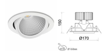
COB 4200 [K] MEAT WHITE Light colour CRI 90 Led chip flux 3539 [lm] Luminous flux 2831 [lm] System power 37 [W] Luminaire Efficiency 77 [Im/W] Beam angle 60° Controller ON/OFF MacAdam 3 SDCM
