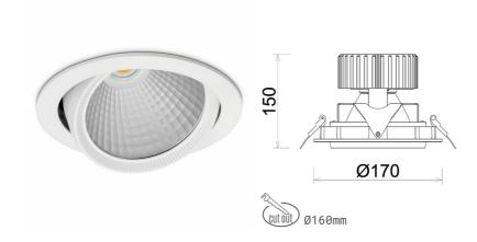
COB 4200 [K] MEAT WHITE Light colour CRI 90 Led chip flux 1412 [lm] Luminous flux 1129 [lm] System power 14 [W] Luminaire Efficiency 81 [lm/W] Beam angle 60° Controller ON/OFF MacAdam
