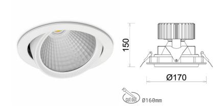
COB 4200 [K] MEAT WHITE Light colour CRI 90 Led chip flux 2340 [lm] Luminous flux 1872 [lm] System power 23 [W] Luminaire Efficiency 81 [lm/W] Beam angle 45° Controller ON/OFF MacAdam 3 SDCM
