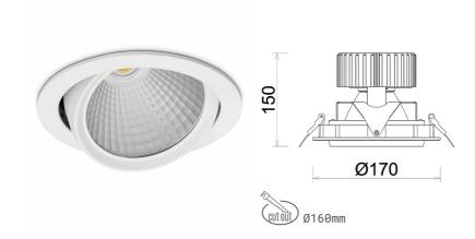
COB 4200 [K] MEAT WHITE Light colour CRI 90 Led chip flux 2159 [lm] Luminous flux 1727 [lm] System power 21 [W] Luminaire Efficiency 82 [lm/W] Beam angle 45° Controller ON/OFF MacAdam 3 SDCM
