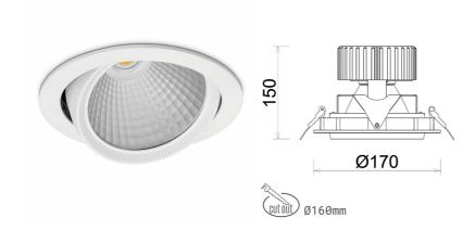
COB 4000 [K] HI EFFICIENT Light colour CRI 90 Led chip flux 4964 [lm] Luminous flux 3971 [lm] System power 31 [W] Luminaire Efficiency 128 [lm/W] Beam angle 60° Controller ON/OFF MacAdam 3 SDCM
