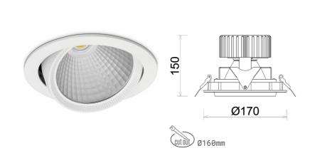
COB 4000 [K] HI EFFICIENT Light colour CRI 90 Led chip flux 3189 [lm] Luminous flux 2551 [lm] System power 19 [W] Luminaire Efficiency 134 [lm/W] Beam angle 45° Controller ON/OFF MacAdam 3 SDCM
