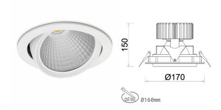
COB 4000 [K] HI EFFICIENT Light colour CRI 90 Led chip flux 4385 [lm] Luminous flux 3508 [lm] System power 27 [W] Luminaire Efficiency 130 [lm/W] Beam angle 30° Controller ON/OFF MacAdam 3 SDCM
