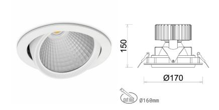
COB 4000 [K] HI EFFICIENT Light colour CRI 90 Led chip flux 3492 [lm] Luminous flux 2793 [lm] System power 21 [W] Luminaire Efficiency 133 [lm/W] Beam angle 15° Controller ON/OFF MacAdam 3 SDCM
