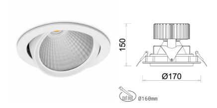
COB 3500 [K] HI EFFICIENT Light colour CRI 90 Led chip flux 3341 [lm] Luminous flux 2672 [lm] System power 21 [W] Luminaire Efficiency 127 [lm/W] Beam angle 30° Controller ON/OFF MacAdam 3 SDCM
