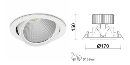
COB 3500 [K] HI EFFICIENT Light colour CRI 90 Led chip flux 3054 [lm] Luminous flux 2443 [lm] System power 19 [W] Luminaire Efficiency 129 [lm/W] Beam angle 30° Controller ON/OFF MacAdam 3 SDCM
