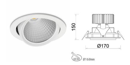
COB 3500 [K] HI EFFICIENT Light colour CRI 90 Led chip flux 1571 [lm] Luminous flux 1256 [lm] System power 10 [W] Luminaire Efficiency 126 [lm/W] Beam angle 30° Controller ON/OFF MacAdam 3 SDCM
