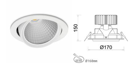
COB 3000 [K] HI EFFICIENT Light colour CRI 90 Led chip flux 2256 [lm] Luminous flux 1804 [lm] System power 14 [W] Luminaire Efficiency 129 [lm/W] Beam angle 60° Controller ON/OFF MacAdam 3 SDCM
