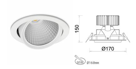
COB 3000 [K] HI EFFICIENT Light colour CRI 90 Led chip flux 5523 [lm] Luminous flux 4418 [lm] System power 34 [W] Luminaire Efficiency 130 [lm/W] Beam angle 45° Controller ON/OFF MacAdam 3 SDCM
