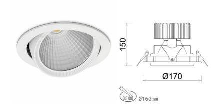
COB 3000 [K] HI EFFICIENT Light colour CRI 90 Led chip flux 5801 [lm] Luminous flux 4640 [lm] System power 36 [W] Luminaire Efficiency 129 [lm/W] Beam angle 15° Controller ON/OFF MacAdam 3 SDCM
