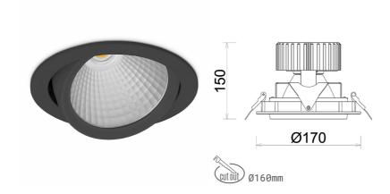
COB 2500 [K] BREAD Light colour CRI Led chip flux 4073 [lm] Luminous flux 3258 [lm] System power 35 [W] Luminaire Efficiency 93 [lm/W] Beam angle 60° Controller ON/OFF MacAdam 3 SDCM
