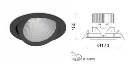
COB 2000 [K] MEAT PINK Light colour CRI Led chip flux 2807 [lm] Luminous flux 2245 [lm] System power 35 [W] Luminaire Efficiency 64 [lm/W] Beam angle 15° Controller ON/OFF MacAdam 3 SDCM
