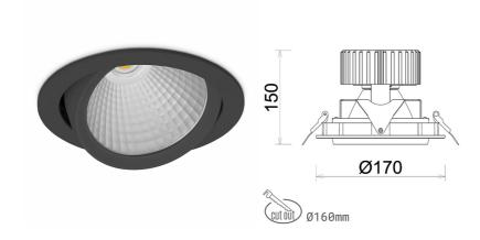
COB Light colour 3000 [K] | CRI Led chip flux 1152 [lm] Luminous flux 921 [lm] System power 10 [W] Luminaire Efficiency 92 [lm/W] Beam angle 45° Controller ON/OFF MacAdam 3 SDCM
