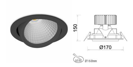
COB Light colour 2700 [K] | CRI Led chip flux 2222 [lm] Luminous flux 1777 [lm] System power 19 [W] Luminaire Efficiency 94 [lm/W] Beam angle 60° Controller ON/OFF MacAdam 3 SDCM
