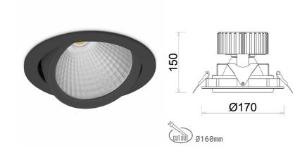
COB Light colour 5000 [K] | CRI Led chip flux 2895 [lm] Luminous flux 2316 [lm] System power 19 [W] Luminaire Efficiency 122 [lm/W] Beam angle 15° Controller ON/OFF MacAdam 3 SDCM
