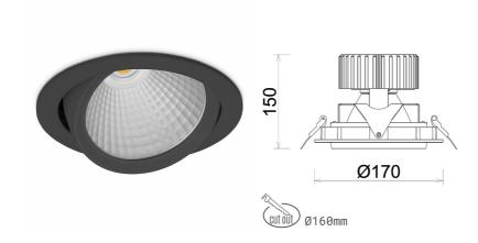
COB Light colour 4000 [K] | CRI Led chip flux 3690 [lm] Luminous flux 2952 [lm] System power 25 [W] Luminaire Efficiency 118 [lm/W] Beam angle 60° Controller ON/OFF MacAdam 3 SDCM
