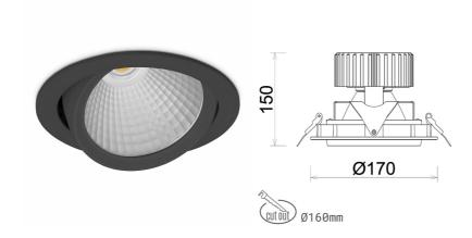
COB Light colour 4000 [K] | CRI Led chip flux 1987 [lm] Luminous flux 1589 [lm] System power 14 [W] Luminaire Efficiency 114 [lm/W] Beam angle 45° Controller ON/OFF MacAdam 3 SDCM
