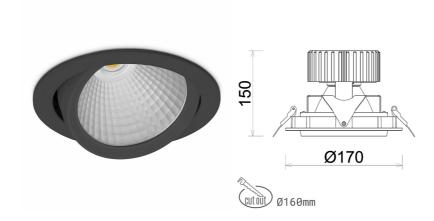
COB Light colour 3500 [K] | CRI Led chip flux 1391 [lm] Luminous flux 1112 [lm] System power 10 [W] Luminaire Efficiency 111 [lm/W] Beam angle 60° Controller ON/OFF MacAdam 3 SDCM
