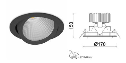
COB Light colour 3000 [K] | CRI Led chip flux 4900 [lm] Luminous flux 3920 [lm] System power 35 [W] Luminaire Efficiency 112 [lm/W] Beam angle 15° Controller ON/OFF MacAdam 3 SDCM
