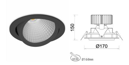
COB Light colour 2700 [K] | CRI Led chip flux 5119 [lm] Luminous flux 4095 [lm] System power 37 [W] Luminaire Efficiency 111 [lm/W] Beam angle 45° Controller ON/OFF MacAdam 3 SDCM
