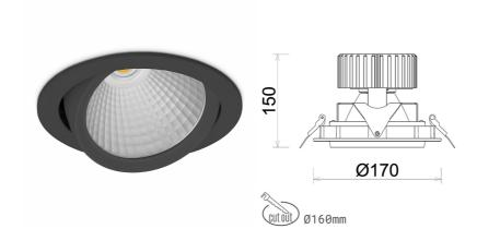
COB Light colour 2700 [K] | CRI Led chip flux 3772 [lm] Luminous flux 3017 [lm] System power 27 [W] Luminaire Efficiency 112 [lm/W] Beam angle 15° Controller ON/OFF MacAdam 3 SDCM
