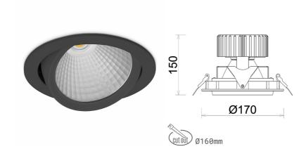
COB Light colour 2700 [K] | CRI Led chip flux 1886 [lm] Luminous flux 1508 [lm] System power 13 [W] Luminaire Efficiency 116 [lm/W] Beam angle 15° Controller ON/OFF MacAdam 3 SDCM
