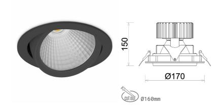
COB 3000 [K] CRI97 Light colour CRI Led chip flux 3915 [lm] Luminous flux 3132 [lm] System power 37 [W] Luminaire Efficiency 85 [lm/W] 30° Beam angle Controller ON/OFF MacAdam 3 SDCM
