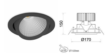
COB 4200 [K] MEAT WHITE Light colour CRI 90 Led chip flux 3375 [lm] Luminous flux 2700 [lm] System power 35 [W] Luminaire Efficiency 77 [Im/W] Beam angle 30° Controller ON/OFF MacAdam
