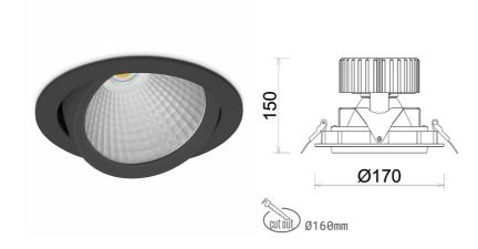
COB 4200 [K] MEAT WHITE Light colour CRI 90 Led chip flux 1412 [lm] Luminous flux 1129 [lm] System power 14 [W] Luminaire Efficiency 81 [lm/W] Beam angle 30° Controller ON/OFF MacAdam 3 SDCM
