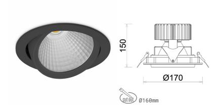
COB 4000 [K] HI EFFICIENT Light colour CRI 90 Led chip flux 3793 [lm] Luminous flux 3034 [lm] System power 23 [W] Luminaire Efficiency 132 [lm/W] Beam angle 45° Controller ON/OFF MacAdam 3 SDCM
