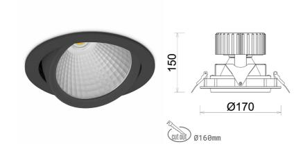
COB 4000 [K] HI EFFICIENT Light colour CRI 90 Led chip flux 4385 [lm] Luminous flux 3508 [lm] System power 27 [W] Luminaire Efficiency 130 [lm/W] Beam angle 15° Controller ON/OFF MacAdam 3 SDCM
