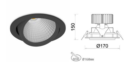
COB 3500 [K] HI EFFICIENT Light colour CRI 90 Led chip flux 3904 [lm] Luminous flux 3123 [lm] System power 25 [W] Luminaire Efficiency 125 [lm/W] Beam angle 60° Controller ON/OFF MacAdam 3 SDCM
