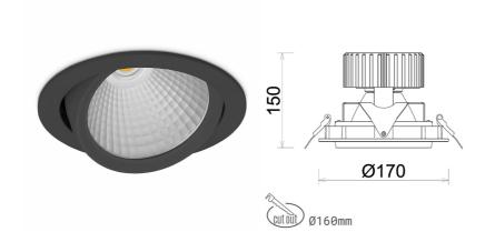
COB 3000 [K] HI EFFICIENT Light colour CRI 90 Led chip flux 5801 [lm] Luminous flux 4640 [lm] System power 36 [W] Luminaire Efficiency 129 [lm/W] Beam angle 60° Controller ON/OFF MacAdam 3 SDCM
