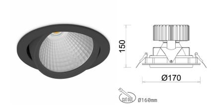
COB 3000 [K] HI EFFICIENT Light colour CRI 90 Led chip flux 3487 [lm] Luminous flux 2789 [lm] System power 21 [W] Luminaire Efficiency 133 [lm/W] Beam angle 60° Controller ON/OFF MacAdam 3 SDCM
