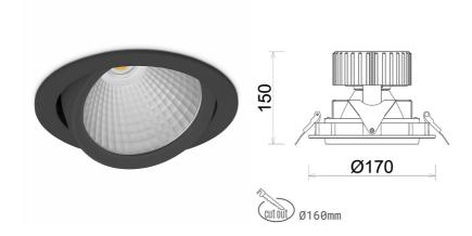
COB 3000 [K] HI EFFICIENT Light colour CRI 90 Led chip flux 4956 [lm] Luminous flux 3964 [lm] System power 31 [W] Luminaire Efficiency 128 [lm/W] Beam angle 15° Controller ON/OFF MacAdam 3 SDCM
