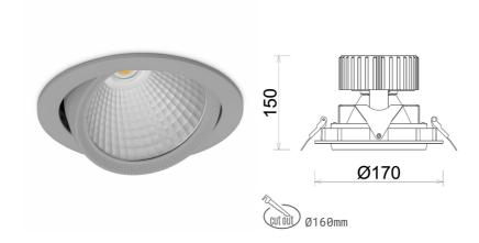
COB 2500 [K] BREAD Light colour CRI Led chip flux 4299 [lm] Luminous flux 3439 [lm] System power 37 [W] Luminaire Efficiency 93 [lm/W] Beam angle 45° Controller ON/OFF MacAdam 3 SDCM
