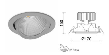
COB 2500 [K] BREAD Light colour CRI 2808 [lm] Led chip flux Luminous flux 2246 [lm] System power 23 [W] Luminaire Efficiency 98 [lm/W] Beam angle 15° Controller ON/OFF
