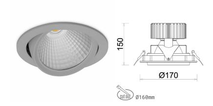
COB 2000 [K] MEAT PINK Light colour CRI Led chip flux 2013 [lm] Luminous flux 1610 [lm] System power 23 [W] Luminaire Efficiency 70 [lm/W] Beam angle 45° Controller ON/OFF MacAdam 3 SDCM
