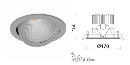
COB 2000 [K] MEAT PINK Light colour CRI Led chip flux 1741 [lm] Luminous flux 1392 [lm] System power 19 [W] Luminaire Efficiency 73 [Im/W] Beam angle 15° Controller ON/OFF MacAdam 3 SDCM
