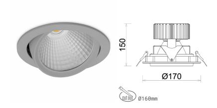
COB Light colour 3000 [K] | CRI 4380 [lm] Led chip flux Luminous flux 3504 [lm] System power 37 [W] Luminaire Efficiency 95 [lm/W] Beam angle 60° Controller ON/OFF MacAdam 3 SDCM
