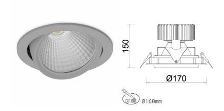
COB Light colour 3000 [K] | CRI Led chip flux 2997 [lm] Luminous flux 2397 [lm] System power 25 [W] Luminaire Efficiency 96 [lm/W] Beam angle 60° Controller ON/OFF MacAdam 3 SDCM
