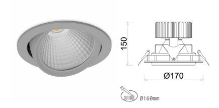
COB Light colour 2700 [K] | CRI 2888 [lm] Led chip flux Luminous flux 2310 [lm] System power 25 [W] Luminaire Efficiency 92 [lm/W] 30° Beam angle Controller ON/OFF MacAdam 3 SDCM
