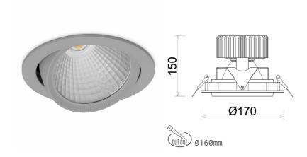
COB Light colour 5000 [K] | CRI Led chip flux 3764 [lm] Luminous flux 3011 [lm] System power 25 [W] Luminaire Efficiency 120 [lm/W] Beam angle 30° Controller ON/OFF MacAdam 3 SDCM
