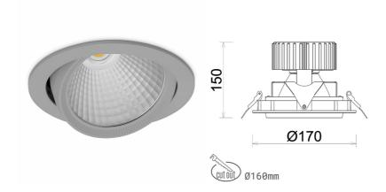
COB Light colour 5000 [K] | CRI Led chip flux 3185 [lm] Luminous flux 2548 [lm] System power 21 [W] Luminaire Efficiency 121 [lm/W] Beam angle 30° Controller ON/OFF MacAdam 3 SDCM
