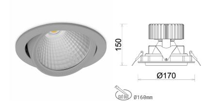
COB Light colour 4000 [K] | CRI Led chip flux 3407 [lm] Luminous flux 2725 [lm] System power 23 [W] Luminaire Efficiency 118 [lm/W] Beam angle 60° Controller ON/OFF MacAdam 3 SDCM
