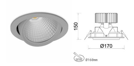
COB Light colour 4000 [K] | CRI 3407 [lm] Led chip flux Luminous flux 2725 [lm] System power 23 [W] Luminaire Efficiency 118 [lm/W] Beam angle 15° Controller ON/OFF MacAdam 3 SDCM
