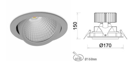
COB Light colour 4000 [K] | CRI Led chip flux 1987 [lm] Luminous flux 1589 [lm] System power 14 [W] Luminaire Efficiency 114 [lm/W] Beam angle 15° Controller ON/OFF MacAdam 3 SDCM
