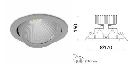
COB Light colour 3500 [K] | CRI 3896 [lm] Led chip flux Luminous flux 3116 [lm] System power 27 [W] Luminaire Efficiency 115 [lm/W] Beam angle 15° Controller ON/OFF MacAdam 3 SDCM
